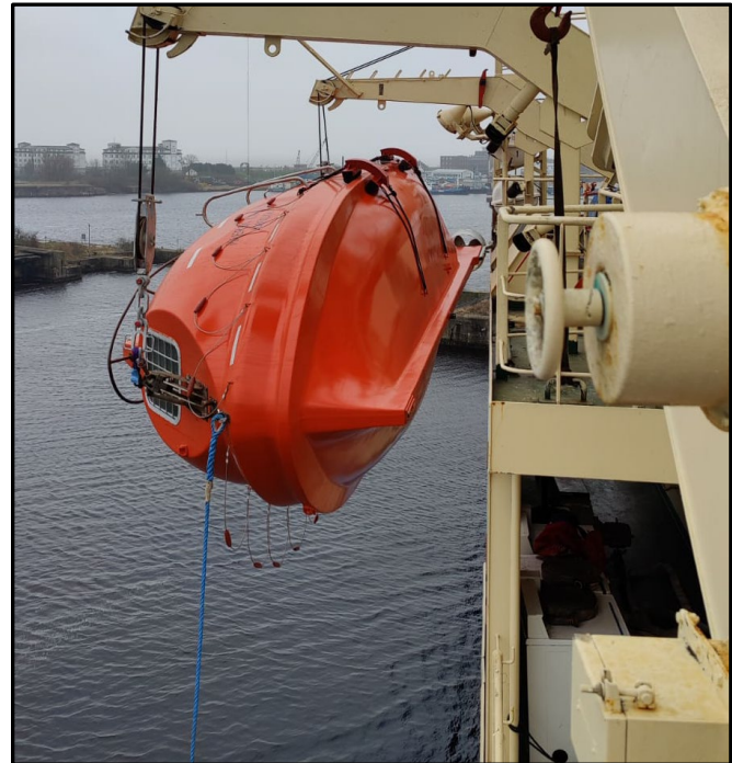
Figure 4 - Lifeboat skeg caught on deck edge.
