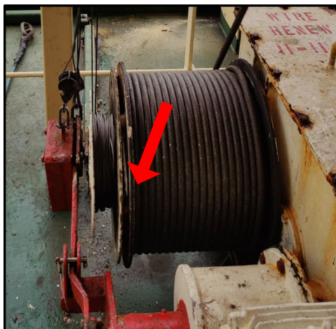
Figure 2 - Poorly-spooled Remote Control Wire.
